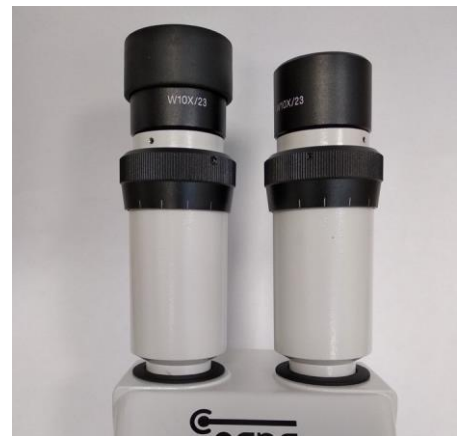
Figure 29 - Dioptre with and without the eyecup
